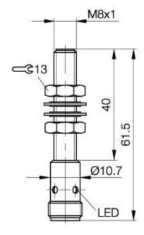
Inductive Sensors BES 516-343-S 4-C M8x1 x 70.5 normally-open Sn=1,5mm shielded
